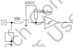
Figure 3-2 Reset Input Port Circuits
