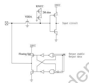
Figure 3-1 General Purpose In/Out Port Circuit.
